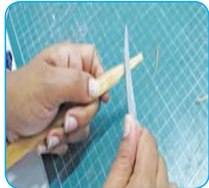
Trim the two edges of the bamboo stick to obtain a tip of 2 mm – 4 mm in width
